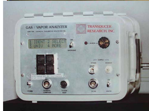
Electronic Nose/CPS100, Stetter, et al. 1985
